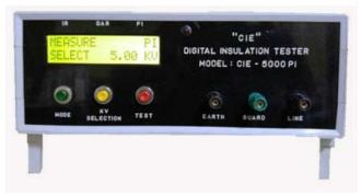
polarization index tests. (Polarisation Index = Resistance after 10 min./Resistance after 1 min.)
